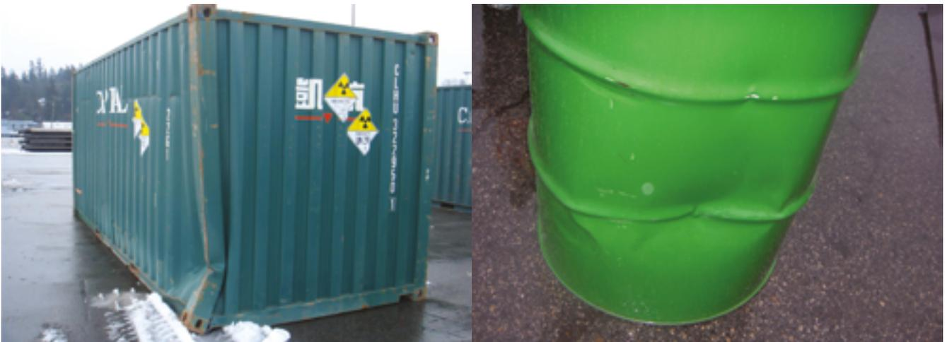
**Figure 9.1: Damage to UOC shipping and packaging containers**
