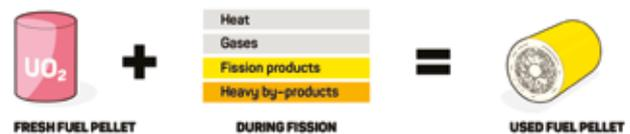
Figure 5.7: The chemical make-up of used fuel
