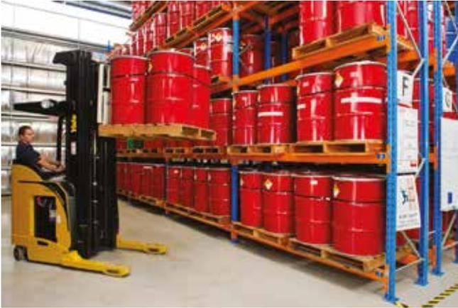
**Figure 5.1: Storage of drums containing low level waste at ANSTO's Lucas Heights facility**
